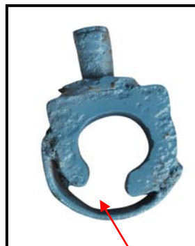
Worn out slot width
