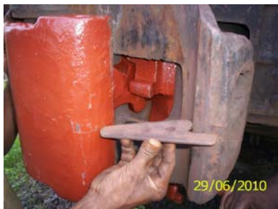
Correct method of gauging
