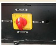
Fig. 18(4) Medha: Isolation switch on top of Onboard Kavach
