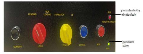
Figure 10: System Indicators on the LP-OCIP
