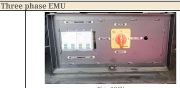
Fig. 18(2) Medha: Isolation switch On onboard Kavach
