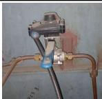
Fig. 19(10) HBL: Diesel loco MR cock at Pn.panel
