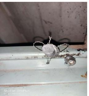
Figure 8: Sealing arrangement in Onboard Kavach
