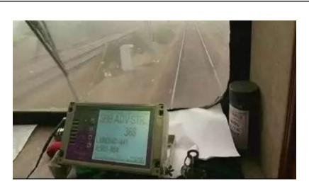
Fig. 2: Fog Safe device being used in train
