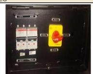
Fig. 17(13) Medha :Two nos. Of MCBs On Onboard Kavach
