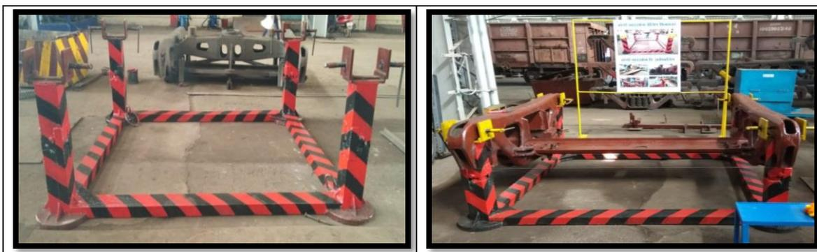
**4. Portable CBC Replacement Gadget at Reception Yard BMY:** For replacement of defective/broken CBC in yard/Sick Line and also in way side stations, 8 -10 men are required with requisite tools & equipment. The activity takes sizable time. A portable CBC gadget was developed at WRC/BMY to ease out the activity and reduce the men and time required.
