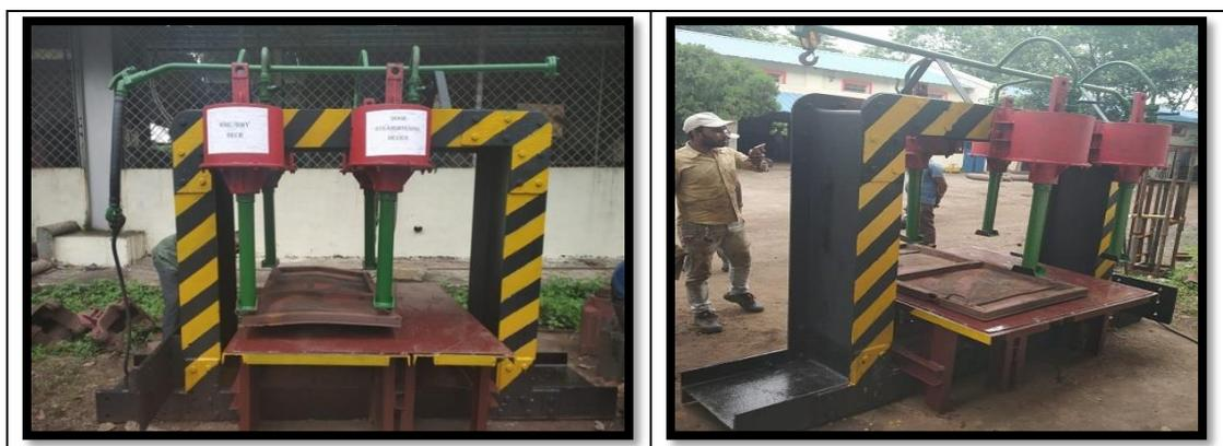
3. **Bogie side frame changing fixture at PP Yard, Bhilai:** In bogie section of PP Yard one side frame changing fixture was developed in house. Defective Trolley parts separated and useable parts assembled for reuse of trolleys with help of this arrangement.
