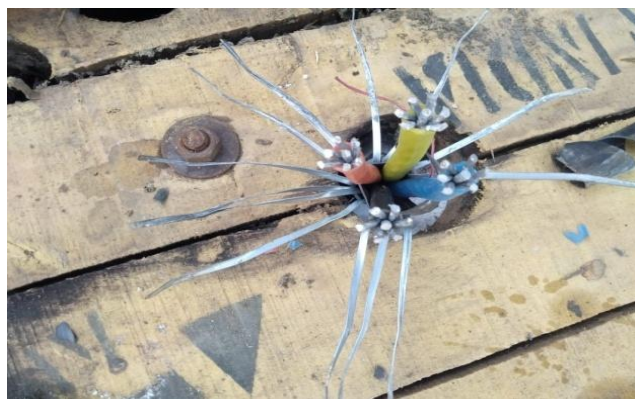
End of cable with 7 strands
