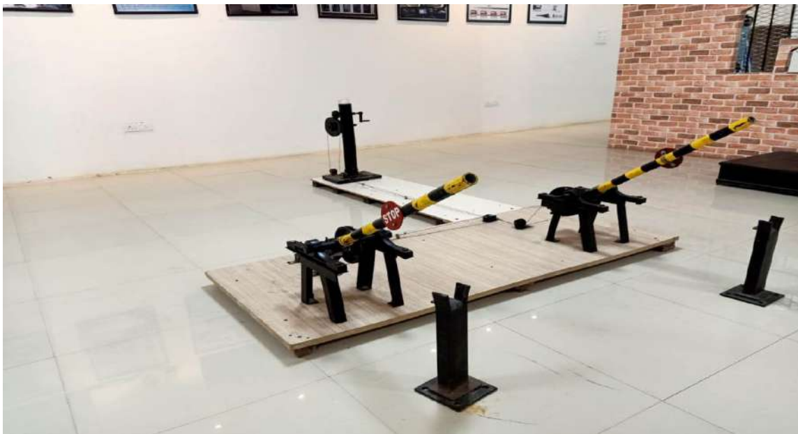
Working model of Signal with Level Crossing gate operation.
