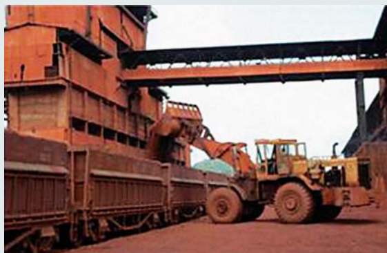
Mechanised loading of iron ore.
