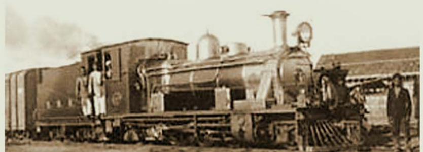
Locomotive number 9 of Raipur Dhamtari Railway(RDR) of Bengal Nagpur Railway(BNR) built by Naysmyth, Wilson & Co. in 1929 was fitted with Stirling superheaters and Lentz Poppet valve gear. Earlier examples were without superheating. Note the headlight that was missing in the non-superheated example seen earlier.
