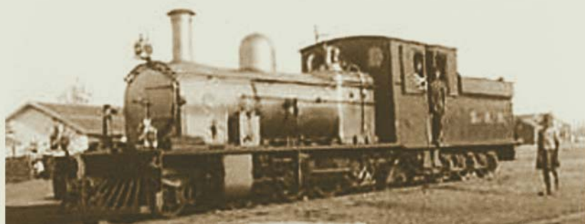
Bengal Nagpur Railway's (BNR) 2-6-2 non superheated locomotives worked exclusively on the Raipur - Dhamtari Railway and later came to be known as RD class engines. Later engines in this series were fitted with Stirling superheaters and Lentz valve gear.
